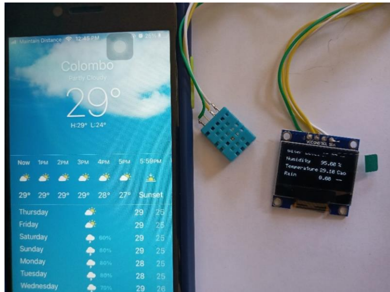
Figure 54: Sensor data reading against actual data
