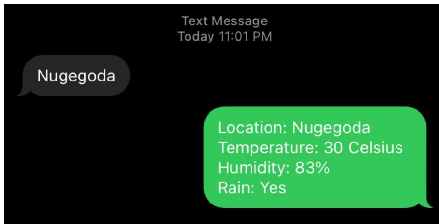
Figure 60: Sample SMS with weather information received upon user request
