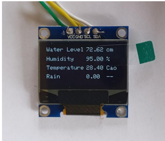
Figure 51: Sensor Data displayed on the OLED screen
